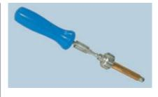
8 Attach the above assembly to the Straight or Offset "T" handle (CES-1-03/04).
