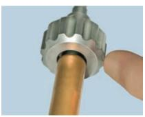
Ensure that the Fluted Nut (CES-SE-13 is assembled so that the Screw Extractor Compression Tube sits in the recess of the Fluted Nut.
