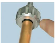
Ensure that the Fluted Nut is assembled so that the Screw Extractor Compression Tube sits in the recess of the Fluted Nut.
