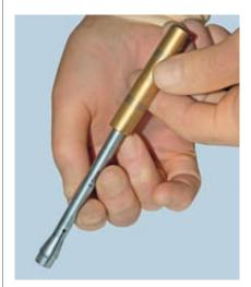
5 Select the corresponding Screw Extractor Shaft (CES-SE-01/14) and slide the Screw Extractor Compression Tube (CES-SE-12) over the Screw Extractor Shaft, followed by the Fluted Nut (CES-SE-13).
