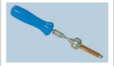
Attach the above assembly to the Straight or Offset "T" handle (CES-1-03/04).
