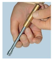
5 Select the corresponding Screw Extractor Shaft (CES-SE-01/14) and slide the Screw Extractor Compression Tube (CES-SE-12) over the Screw Extractor Shaft.
