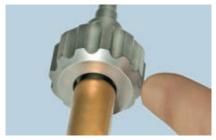
6 Followed by the Fluted Nut (CES-SE-13. Ensure that the Fluted Nut is assembled so that the Screw Extractor Compression Tube sits in the recess of the Fluted Nut.
