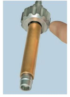
4 Followed by the Fluted Nut (CES-SE-13). Ensure that the Fluted Nut is assembled so that the Screw Extractor Compression Tube sits in the recess of the Fluted Nut.
