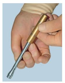
3 Slide the Screw Extractor Compression Tube (CES-SE-12) over the Screw Extractor Shaft.
